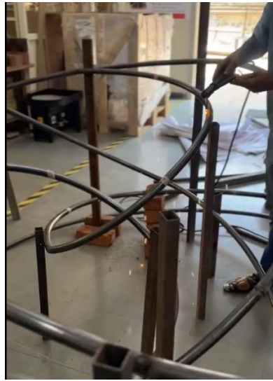
Using the MR for checking the precision and welding the complex assembly
