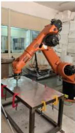
SPIF on a Aluminum sheet @ DFL, BNCA
