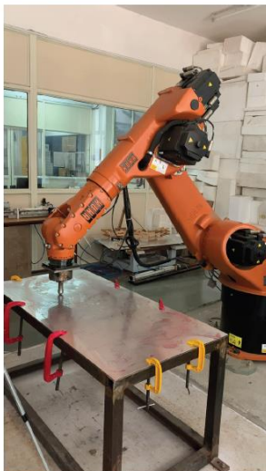
SPIF on a Aluminum sheet @ DFL, BNCA
