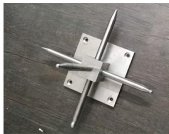
Assembled SPIF tool @ DFL, BNCA
