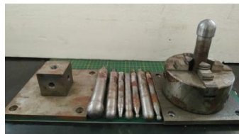
SPIF tool with different tips ranging from 2mm-20mm @ DFL, BNCA
