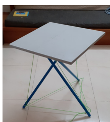
3 strut tensegrity with PVC pipes and nylon rope used as a support for tabletop
