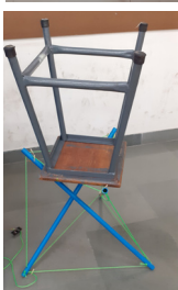
3 strut tensegrity with PVC pipes and nylon rope used as a support for tabletop
