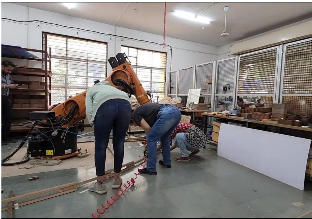
Students interacting with the KUKA pick and place and physically nailing the layers
