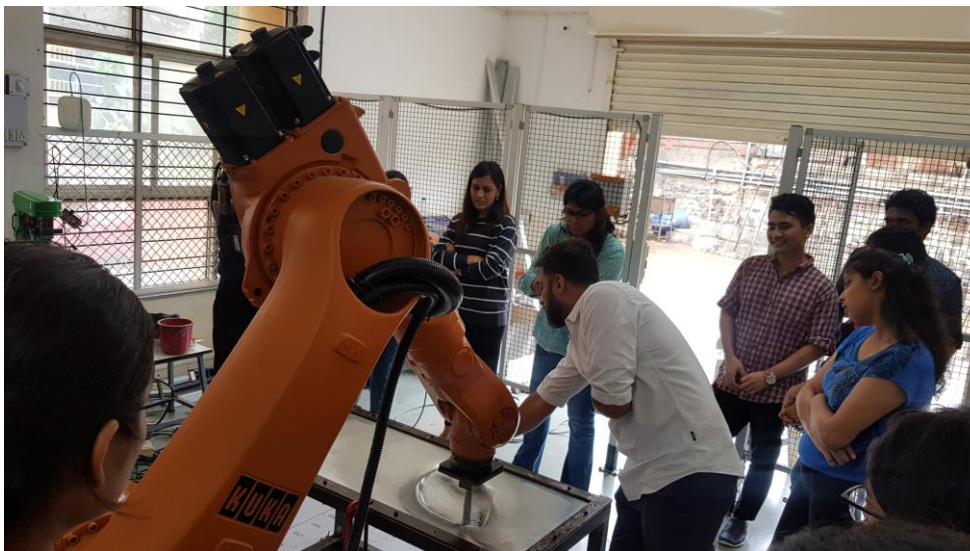
Tutors explaining the sheet deformation (SPIF)
