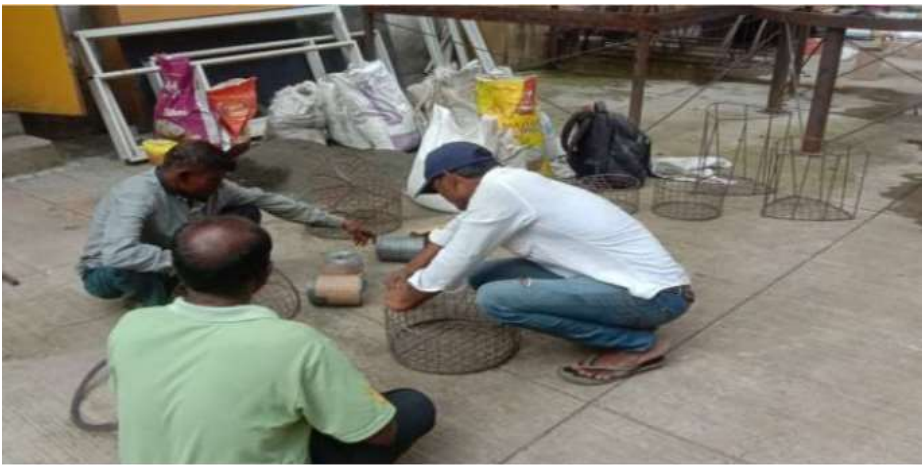
Fabricators preparing moulds for planters
